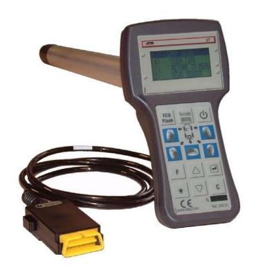
The principle of this instrument is to awaken and then retrieve data from smart valves mounted on vehicle wheels, in order to check their identifiers and/or program the vehicle's onboard computer. This tool is intended for making adjustments on vehicles on the production line, or for programming valves in any company that uses or installs smart valves.
