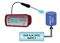
The operator can search for the leak location with the test probe. The device detect and every gas leak with the probe and displays the gas concnetration. External probe method.
