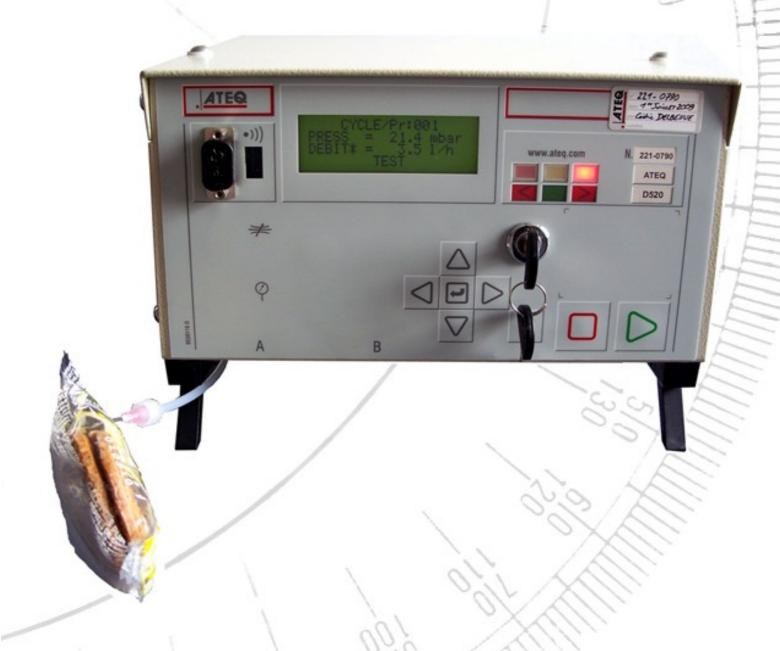
Leak detection measurement without using gas or liquid.
